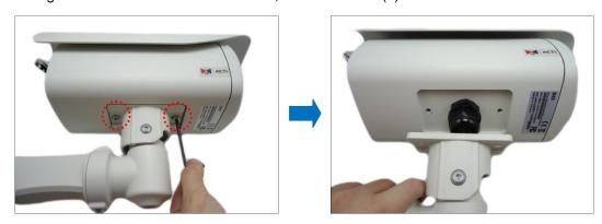
2. Remove the clamping nut and sealing insert.
