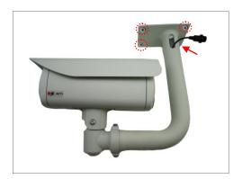
**NOTE:** Screws for ceiling installation are not supplied with the camera nor the ceiling bracket package. Purchase applicable screws separately according to the material of the ceiling where the camera will be installed.
